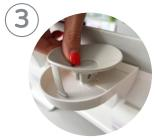
Push the new suction cup onto the housing ensuring that the holes match up.
